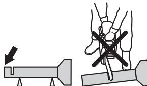
If the pipe is allowed to sag and close the cut, the bar will be pinched in the kick back zone and a severe kick back might develop. If the pipe is properly supported the end of the pipe will move downward, the cut will open and no pinching will occur.
