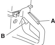
The trigger lock remains pressed in as long as the throttle is pressed. When the grip on the handle is released the throttle trigger and the throttle trigger lock both return to their original positions. This is controlled by two independent return spring systems. This means that the throttle trigger is automatically locked in the idle position.
